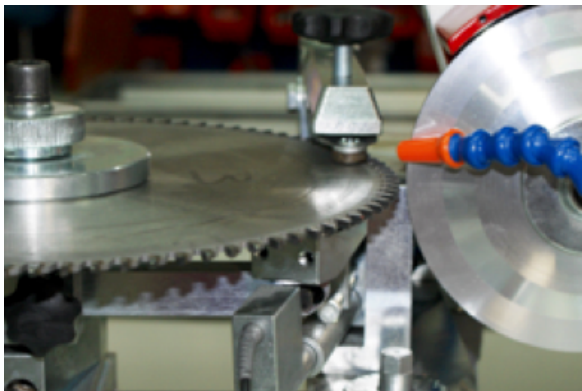
Circular saw blade refrigeration. The machine can be optionally equipped with refrigeration system which includes tray, coolant tank and pump.
