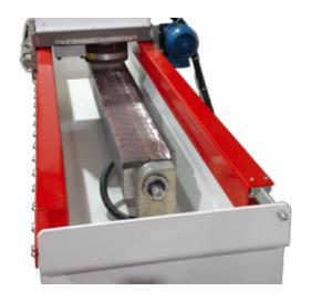
Magnetic chuck 150 mm. width supported by extra rigid feet
