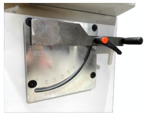
Knife degrees easy and fast to adjust by means of a graduated lever from 0° to 90°
