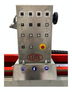
Control panel very easy to use with only the needed buttons just like the old machines, but internally there is a powerful PLC system, so that the sharpening cycle is easy to adjust and automatic
