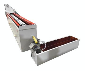
Version with magnetic disc cleaner for automatic removal of magnetizable dirt.
