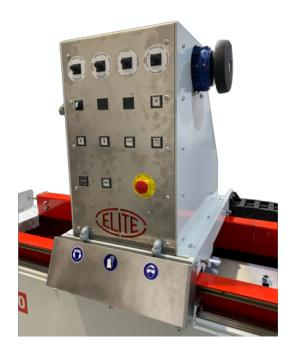
Automatic or manual downfeed of grinding wheel: You can move up or down the grinding wheel with the push buttons, or do it with the manual handwheel to get a more precise feedback
