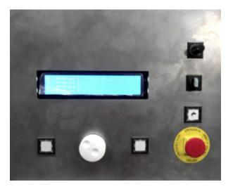
Program your own sharpening parameters with the standard CNC panel. It allows to realize and to save programs, perfect for the sharpening of paper knives or knives manufacturing.
