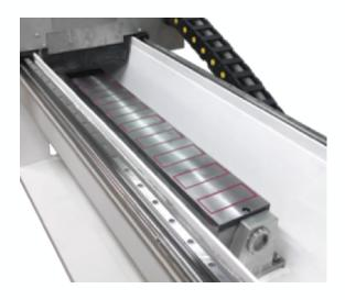
Magnetic knives chuck magnetizable and demagnetizable from the control panel. Same clamping force on the end of the plate or in the center: however narrow the knives are held perfectly on the edge of the plate. The strongest fixing on the market in knives sharpening machines. The super-polarity system is optionally available. With a fixing increased by 20%.
