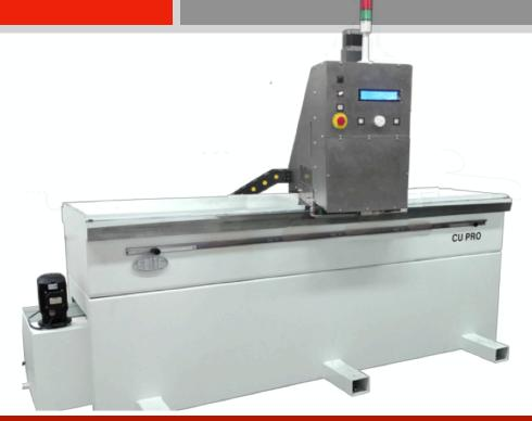
Our ELITE CU PRO model is the most advanced manufacturing and sharpening knives machine. It features a grinding head designed to prevent corrosion better than standard painted grinding heads, equips a direct drive motor: this lets you have 20% more engine power compared to other engines that incorporates belt transmission.
